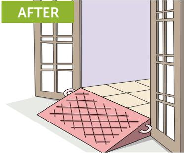
Installation of removable wooden ramp with non-skid covering
