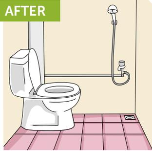
Filling up the step-down shower area with cement and tiles to level the toilet flooring
