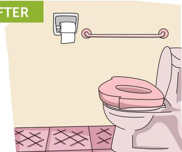
A sitting toilet with an additional toilet raiser, installation of grab bar and anti-slip floor treatment
